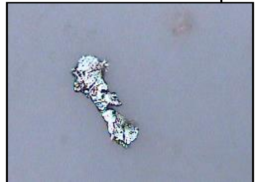
Hard Particle Damaged Metallic Wear Debris. @ 500X Sized 0.2-55 µm Brightfield
